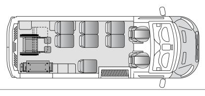
**CHASSIS SPECIFICATIONS:** LONG-EL HIGH Wheelbase: Overall Length: 263.9" Height: 110.4" Width - Excluding Mirrors: 81.3"/83.7" Width - Including Mirrors: 97.4" Width - Mirrors Folded: 83.2"/83.7" Front Track: 68.2"/68.5" Rear Track: 68.6"/65.7" Front Overhang: 40.3" Rear Overhang: 76" Load height (Curb): 28" Rear Cargo Door Opening Height: 74.3"
